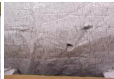
Small puncture in MP Global box liner
